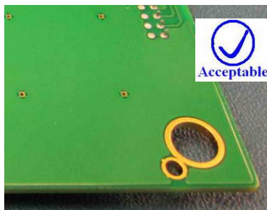
Figures C6-1: No damaged edge 边缘无损伤
