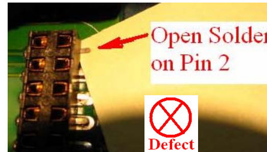
Defect Figure E6-2: Open solder in Pin2 pin2 未焊上
