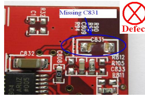
Defect Figure G1-2: Missing C831
