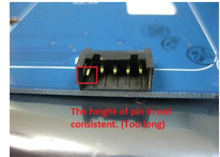
Figure E4-1: 1) Pin height tolerance pin 高度差 2) Less than 50% pin thickness 弯曲少于厚度的一半 Defect Figure E4-2: One Pin was bent pin 弯曲
