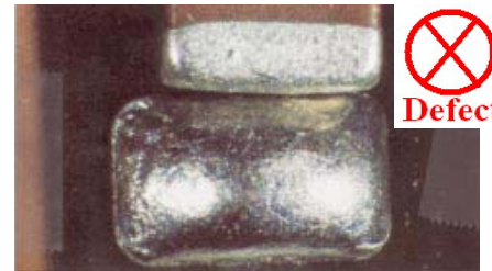
Defect Figure G2-1: Solder has not wetted to the land / termination 元件未与焊盘连接
