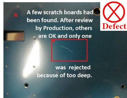
Defect Figure C4-2: Scratch line is too deep 划痕太深
