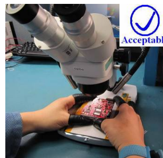
Figure 2: Using 40X microscope to check the soldering status
