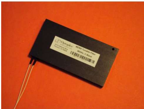
Figure 3a, Photo of a 50GHz MEMS TF full functional module with control electronics included. The size is 104 x 52.5 x 12.5mm.
