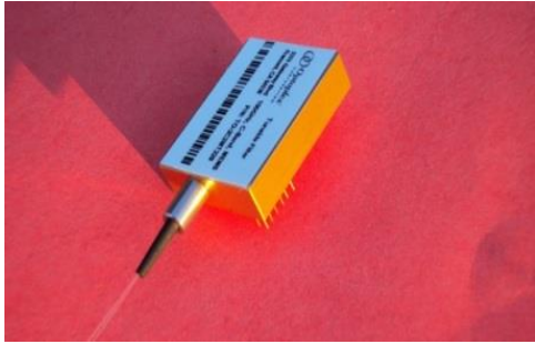
Figure 3a, Photo of a 100GHz MEMS TF (optical engine with analog control interface, no control electronics included). The size is 35 x 25 x 8.5mm.
