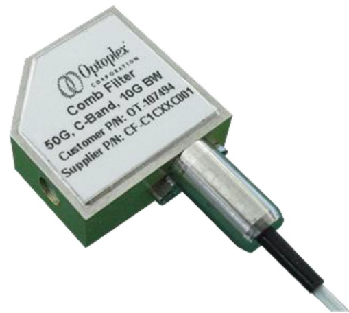
Figure 1.3, Photo of a 50GHz comb filter
